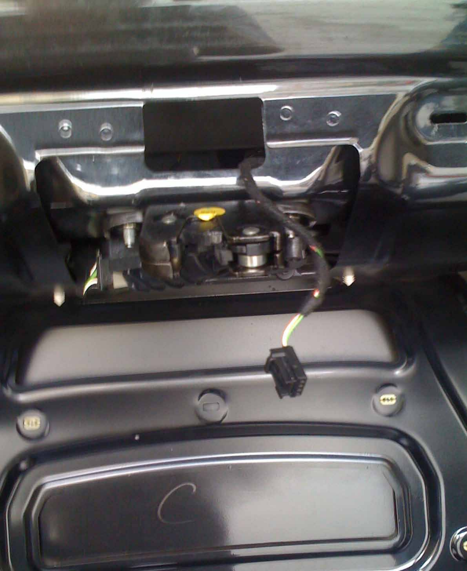
The connector for the button is in place
